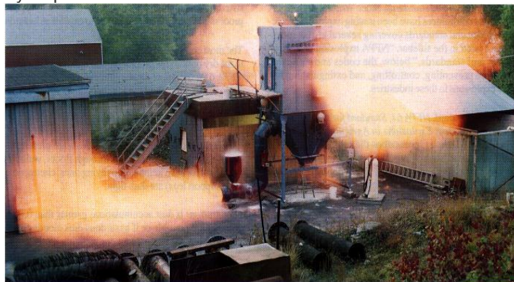
In a test explosion at a combustion research center, a vent panel on a dust collector ruptures to safely vent the explosion. Flashback down the collector's inlet duct (at bottom) illustrates why it's important to incorporate an explosion isolation system between connected process equipment.
